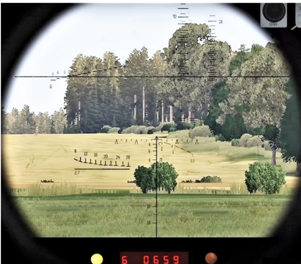
Monitoring of the field of view of the 1G46 sight at the instructor's workstation
