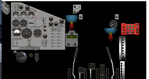
Monitoring of the field of view of the 1G46 sight at the instructor's workstation
