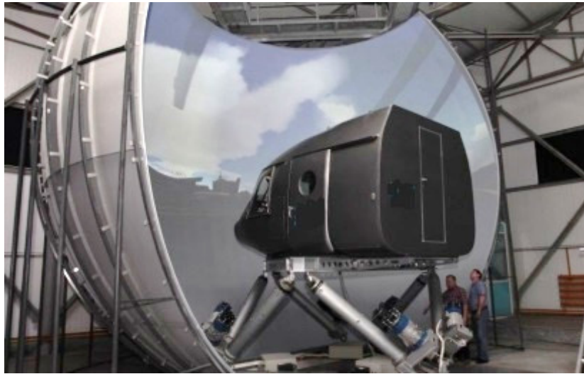
The Cockpit mounted on the motion system and static projection screen
