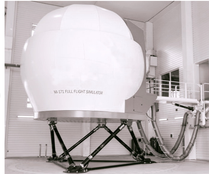
The Cockpit and static projection screen mounted on the motion system
