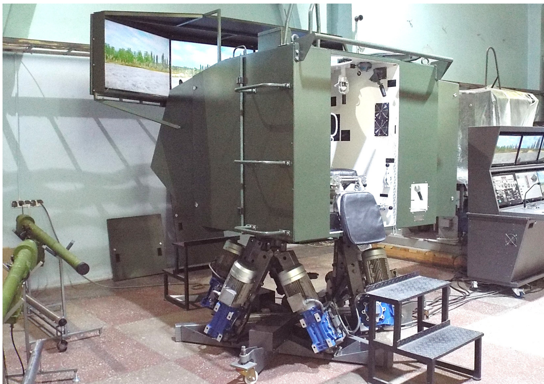
The BMP-3 driver's compartment functional mock-up mounted on a 6DOF dynamic platform
