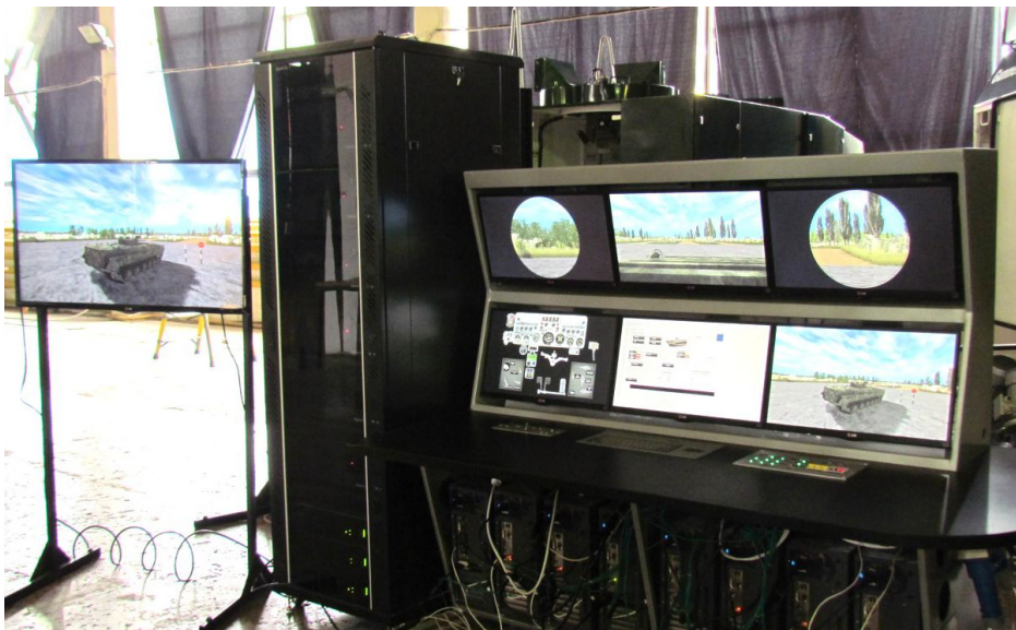
The monitor for supervising the field of view of the SOZH-M sight of the gunner-operator in day mode
