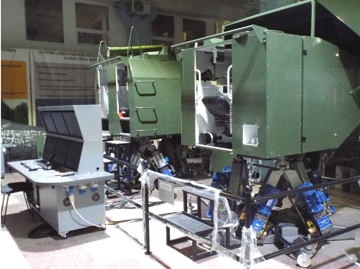
The BMP-3 driver's compartment functional mock-up mounted on a 6DOF dynamic platform
