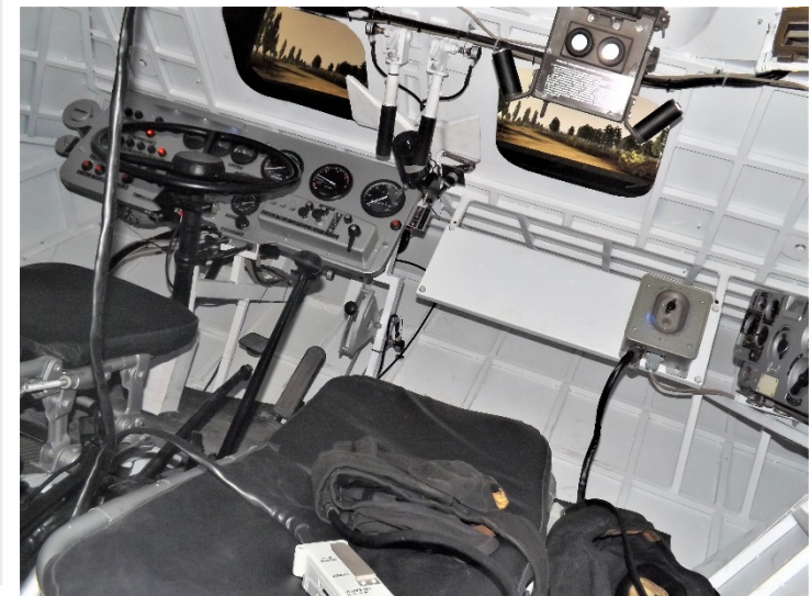
BTR-80 driving compartment interior correspondence
